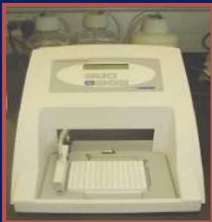
13. Wash Capture plate on plate washer
